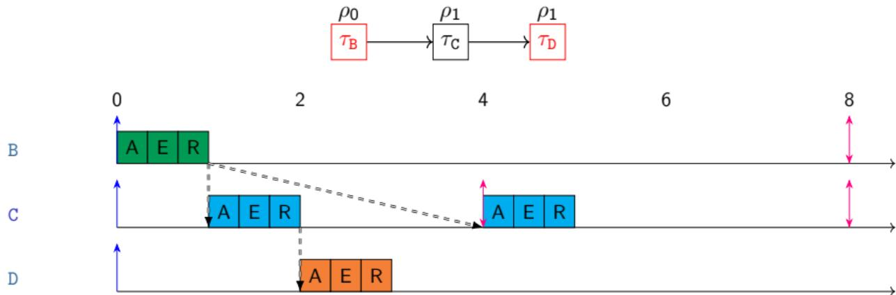
Simplification n°1 : Sensors/Actuators have no A/R phase
