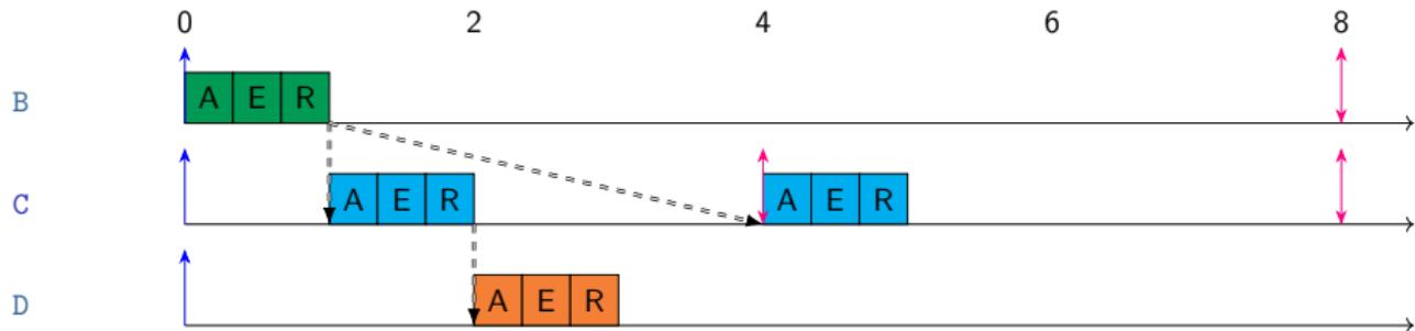
Simplification n°1 : Sensors/Actuators have no A/R phase
